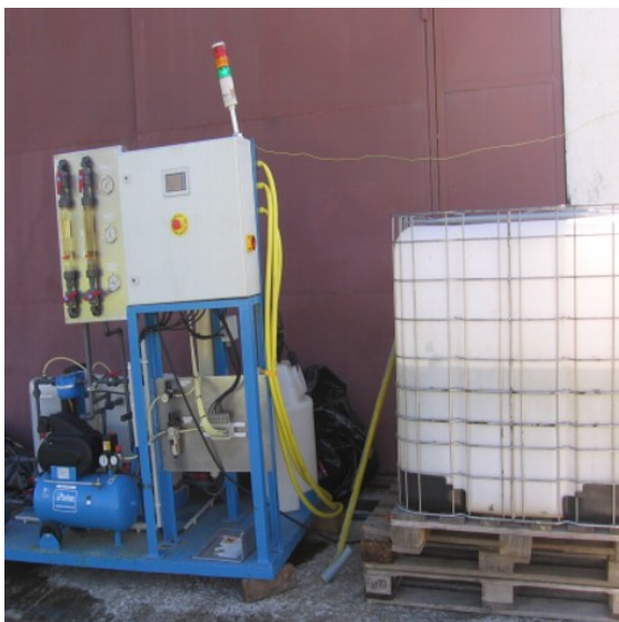
Fig.2. The image of microfiltration-ultrafiltration pilot plant
